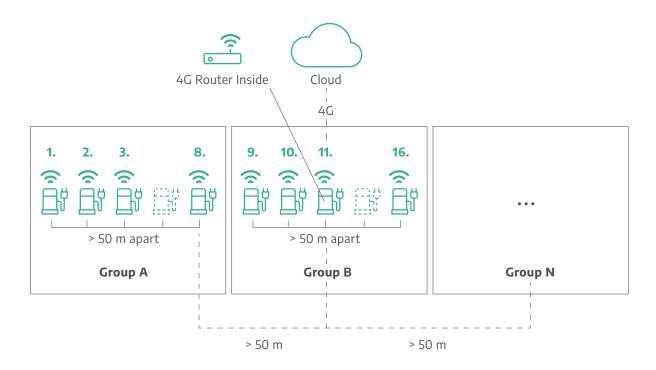
A 4G router is recommended to be installed at the center of all chargers or at a position with the best 4G signal coverage. The 4G router could be supplied by EN+ and it can be installed inside the charger. To keep a stable WiFi connection, the distance between 4G router and the nearest charger should be less than 50 meter. If there are walls or obstacles in between, the distance should be kept less than 20 meter. Same requirement for the distance between two nearby chargers.
